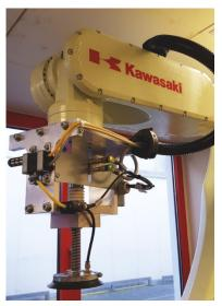
The vacuum gripper reliably picks up the paint buckets.
