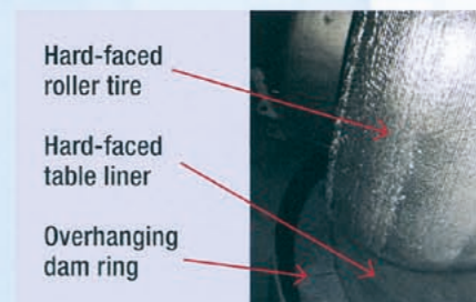
Fig. 2 Hard-faced roller tire and table liner
