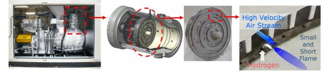
Gas turbine unit and dry low NOx combustor using micro-mix combustion technology
