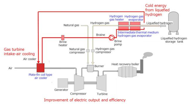
Structure of a gas turbine intake-air cooling system that utilizes cold energy from liquefied hydrogen
