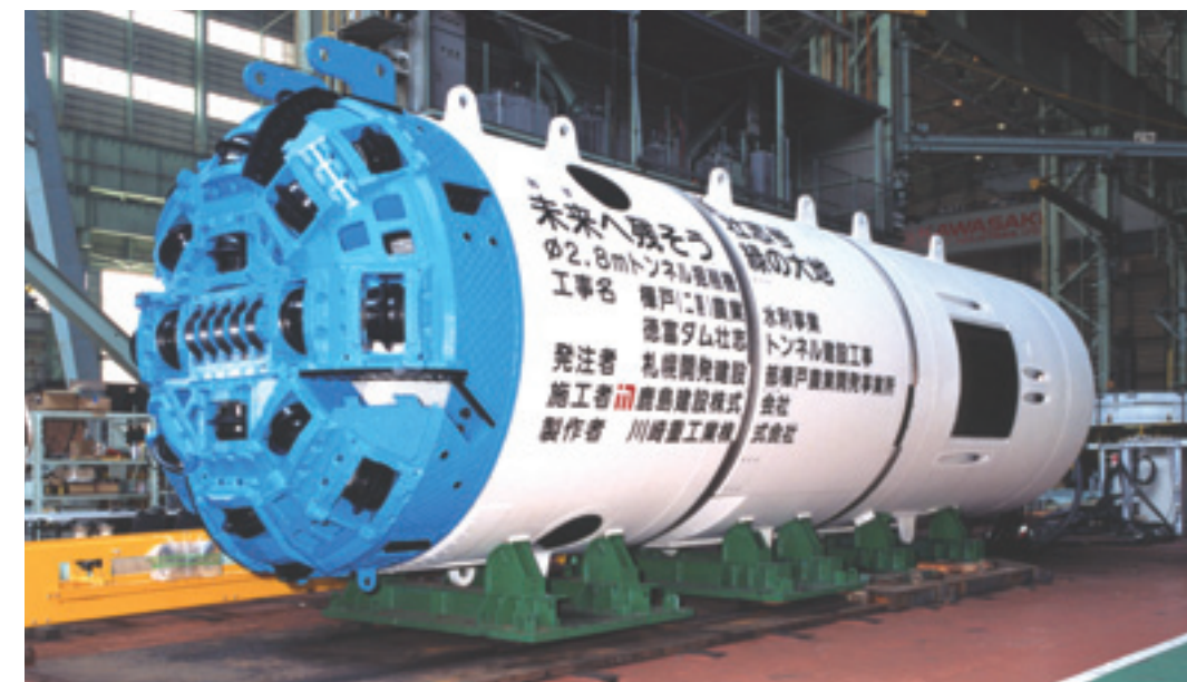
φ2.8m full shield TBM(belt conveyor discharge system)
