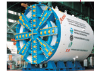
φ7.16m dual-mode earth pressure balanced shield machine (Singapore sewage system, Singapore)
