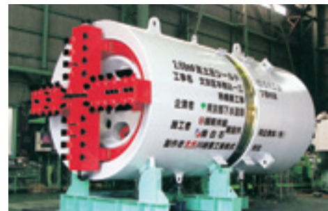
φ2.68m earth pressure balanced shield machine (DSR construction method)
