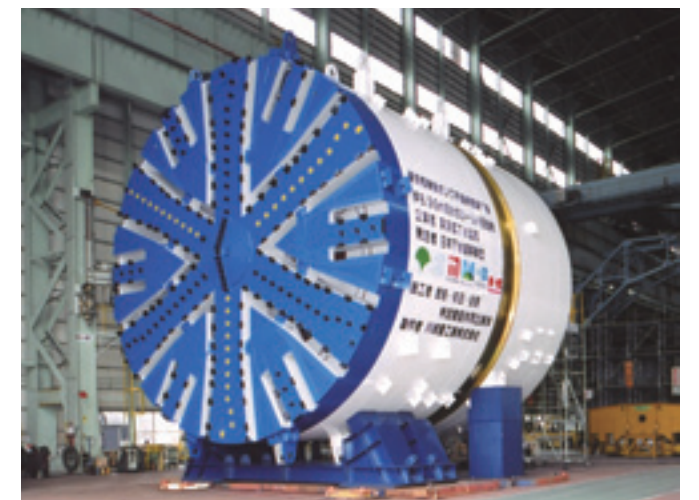
φ8.99m slurry shield machine (Cutter bits exchange device*, For 30 m radius curvat)
