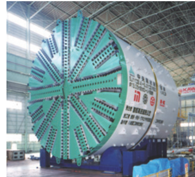
φ13.05m slurry shield machine (Cutter bits exchange device*)
