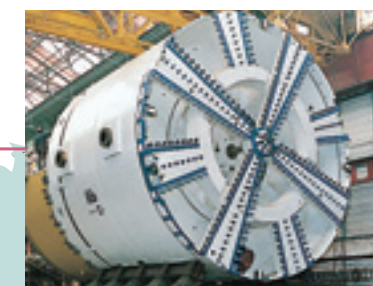
φ7.65m earth pressure balanced shield machine (Lille subway No. 2 Line, France)
