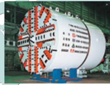
φ6.14m earth pressure balanced shield machine (Guangzhou subway No. 1 Line, China)
