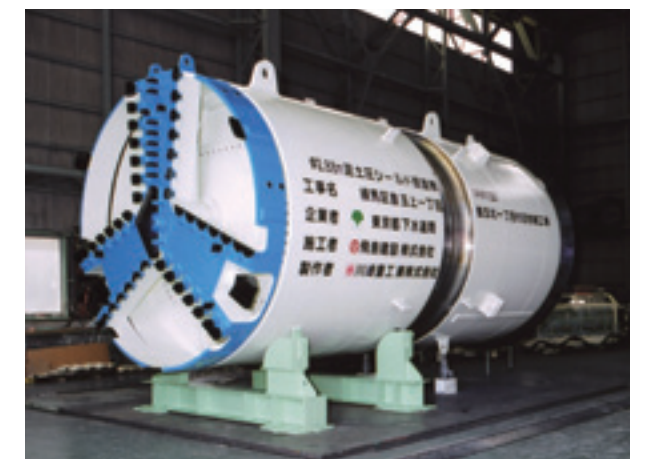
φ2.88m earth pressure balanced shield machine (Excavated 10 mR sharp curvature)
