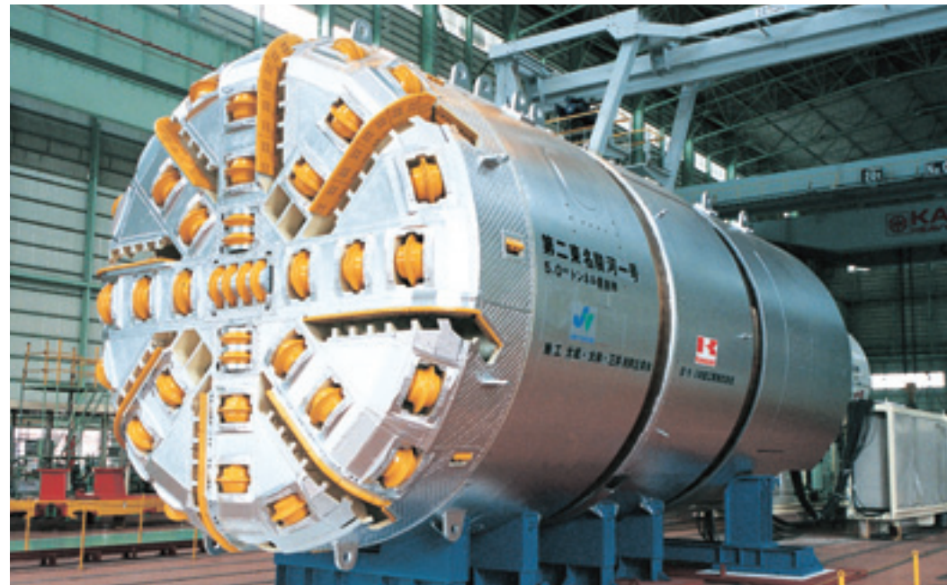
φ5m full shield TBM(30 mR, belt conveyer discharge system)
