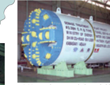
φ3.38m earth pressure balanced shield machine (Malaysia sewage, Malaysia)
