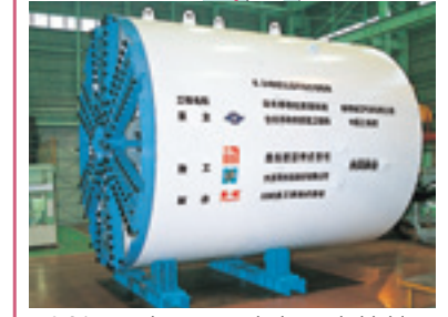
φ6.24m earth pressure balanced shield machine (Taipei subway Nankang Line, Taipei)
