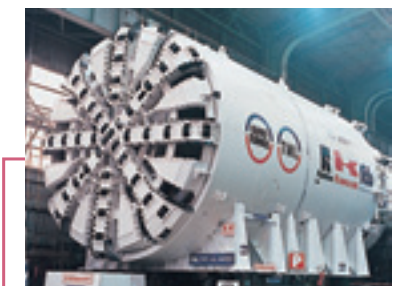
φ8.78m shield TBM (Channel Tunnel Undersea Railroad Project, France)
