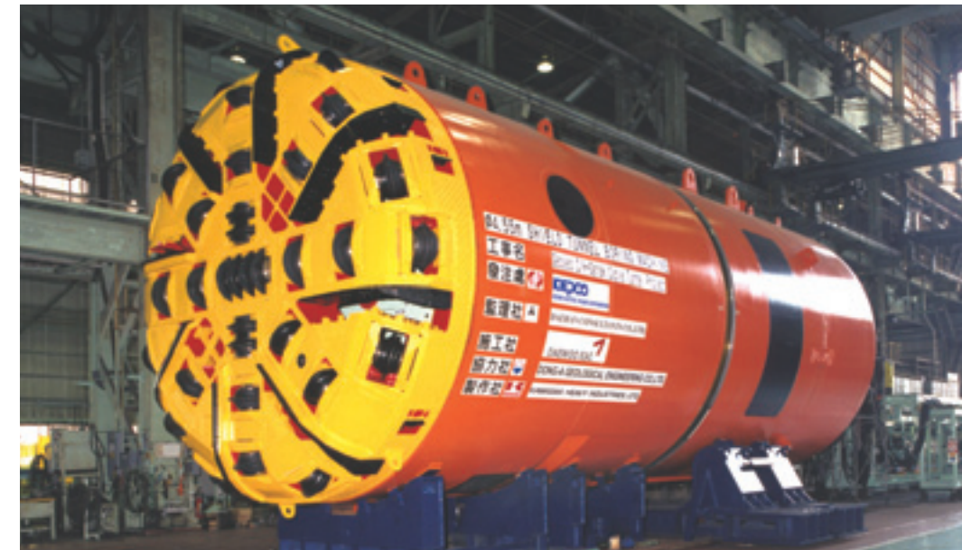
φ4.55m full shield TBM compatible belt conveyer discharge with screw conveyor system. (screw conveyor/belt conveyor discharge system)
