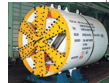
φ6.43m dual-mode earth pressure balanced shield machine (Bangkok subway Blue Line, Thailand)
