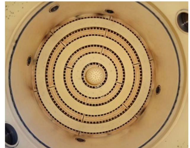
Combustor interior after 2h test
