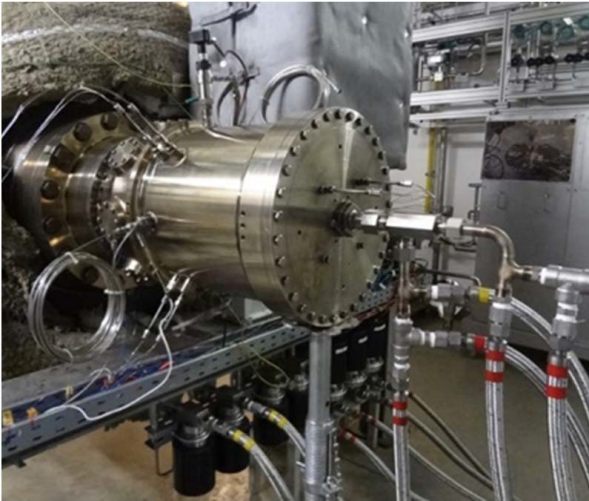
Hydrogen 100% DLE Combustor test in Aachen University of Technology)
