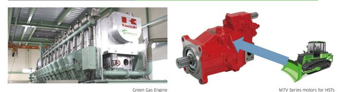
1. HST: Hydrostatic transmission: A non-stage transmission comprising a hydraulic pump and hydraulic motors
