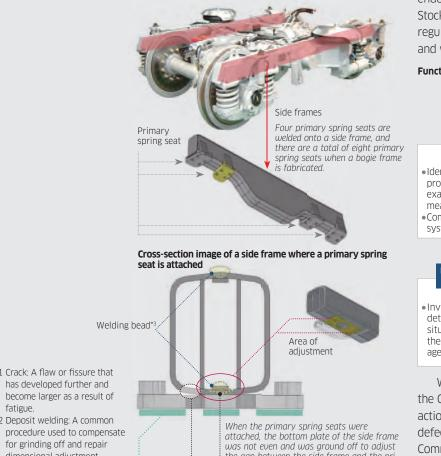
the gap between the side frame and the pri mary spring seat to 0.5mm or less. Gaps between the side frame and the primary
