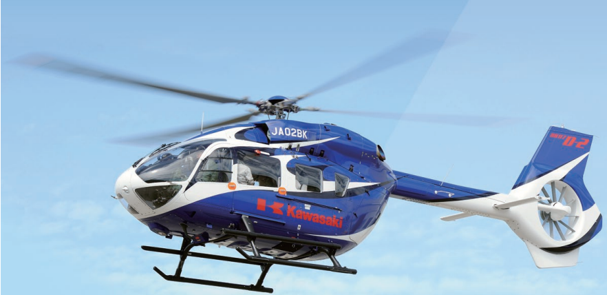
Through introduction of a Fenestron® and increasing the number of blades, higher noise frequency reduces the noise level. In addition, introduction of unequal blade spacing design contributes to further noise reduction due to canceling of harmonic noise peak.
