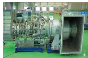
Gas Turbine “L30A”
