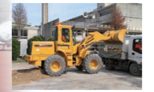
Wheel loaders For clearing and carrying away rubble
