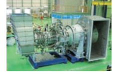
L30A gas turbine
