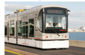
SWIMO: Low-Floor Battery-Powered Light Rail Vehicle (LRV)
