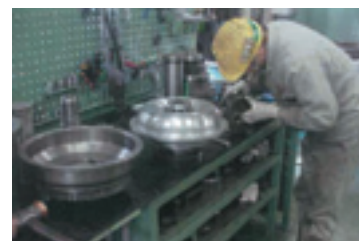
Transmission being restored in the rebuilding process
