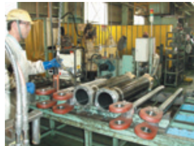
Hoist cylinder manufactured from near net shape
