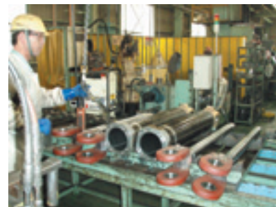
Hoist cylinder manufactured from near net shape
