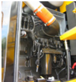
Engine fitted with turbo charger and intercooler
