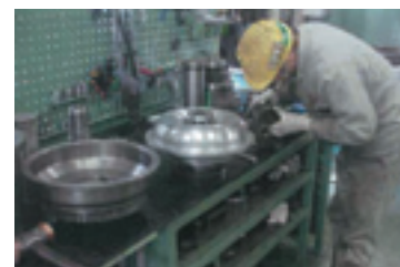
Transmission being restored in the rebuilding process
