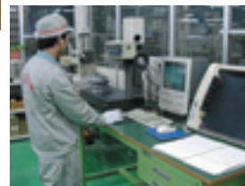
Dimensions measurement and inspection of procured parts
