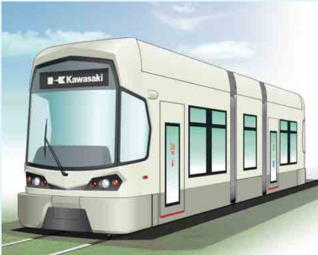
Image of Kawasaki LRV SWIMO which can travel in area without trolley wire
