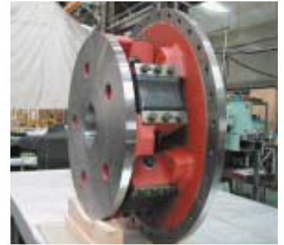
Newly developed KC coupling (Kawasaki compression type elastic coupling)
