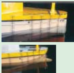
Upper: New bow form (SEA-Arrow) Lower: Conventional bulbous bow
