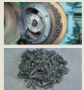
RDF forming machine and RDF
