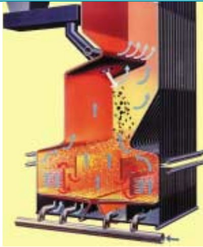
Highly Efficient Internal Circulation Fluidized Bed-type Boiler
