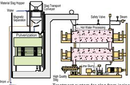
Treatment system for slag from incineration ash
