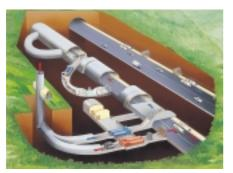
Electrostatic precipitator installed in a road tunnel
