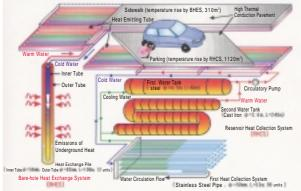
Road surface temperature control system at Hachikita service area. (Snow melting operation)
