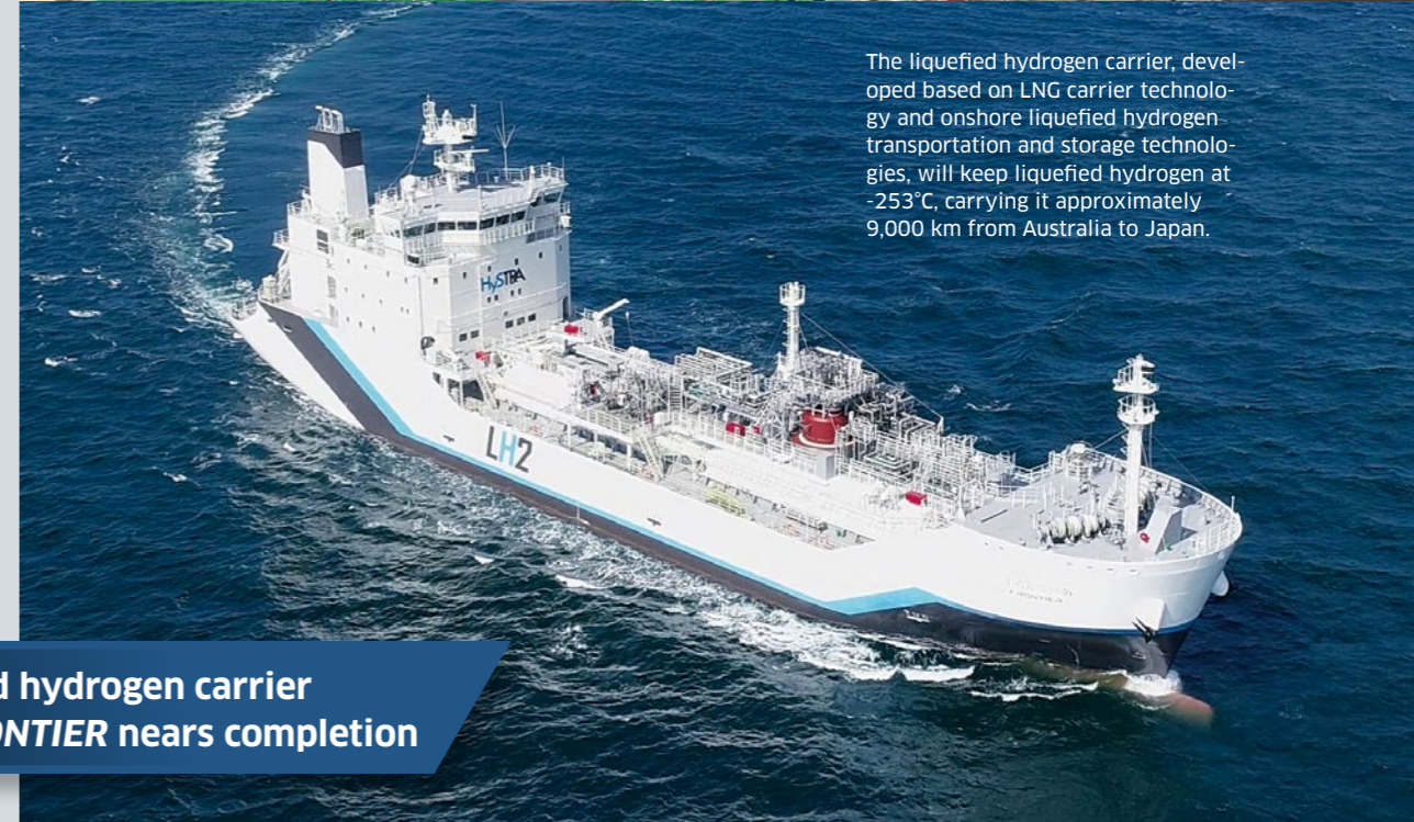
Here, hydrogen will be liquefied and loaded onto the liquefied hydrogen carrier. At -253°C, the liquefied hydrogen's bulk is just one eight-hundredth its volume as a gas, dramatically improving carrying efficiency.
