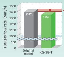
Reducing 41Nm³/h = 3% of fuel gas flow rate
