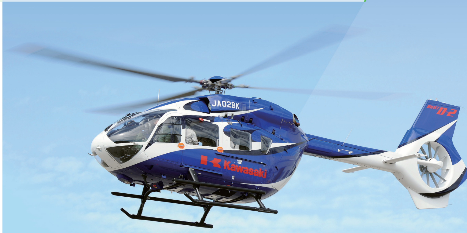
Through introduction of a Fenestron® and increasing the number of blades, higher noise frequency reduces the noise level. In addition, introduction of unequal blade spacing design contributes to further noise reduction due to cancelling of harmonic noise peak.
