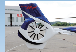
Through introduction of a Fenestron® and increasing the number of blades, higher noise frequency reduces the noise level. In addition, introduction of unequal blade spacing design contributes to further noise reduction due to cancelling of harmonic noise peak.
