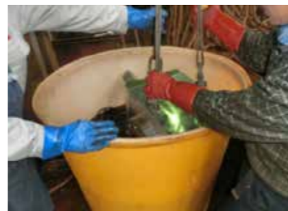
Figure 4: After improvement: Removal of resin using solvents
