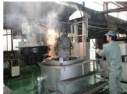
Figure 3: Before improvement: Heating incineration of resin
