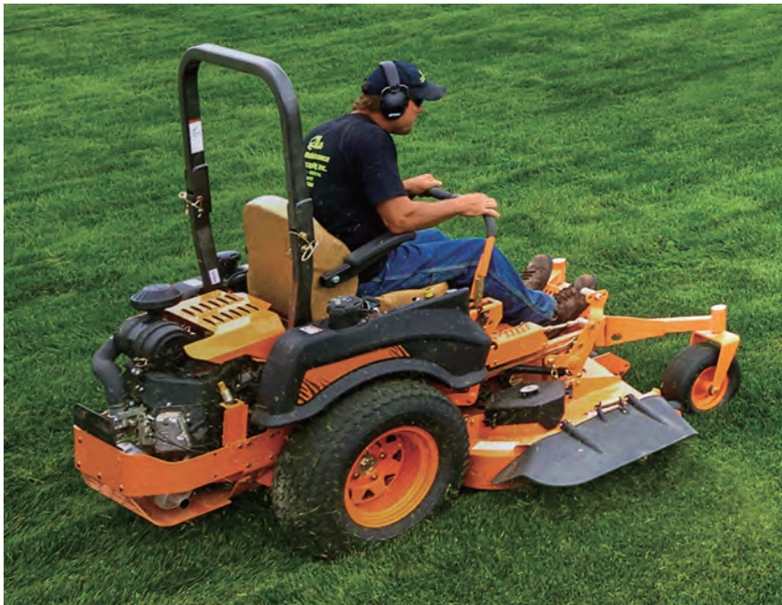
Fig. 2 Riding mower mounted with FX850V-EFI (ZTR)
