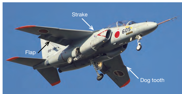
Fig. 6 Aerodynamic devices used for aircraft
