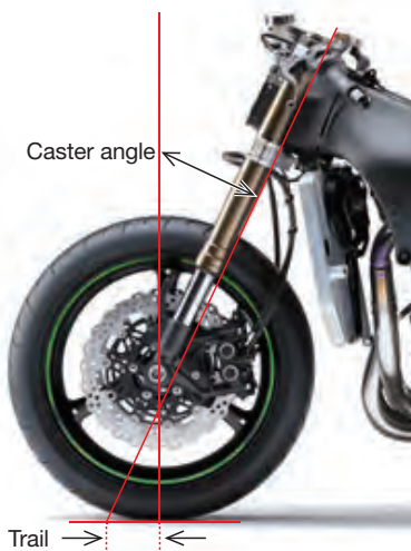
Fig. 1 Caster angle and trail
