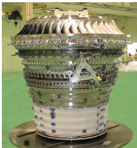
Fig. 3 Appearance of the IPC module
