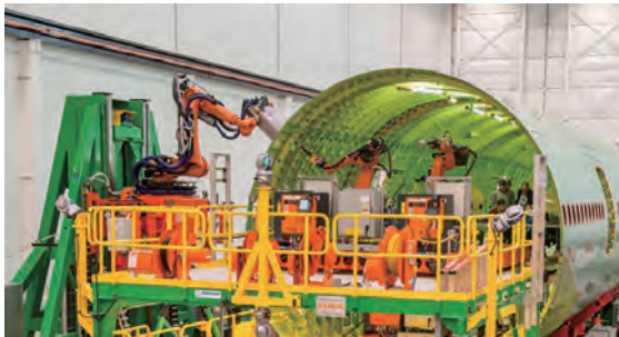
Fig. 4 Final assembly using robots (at Boeing)
