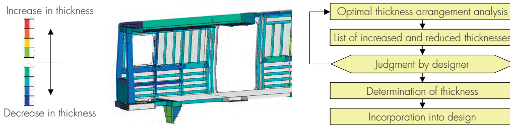
(a) Optimization of the thickness of carbody structures
