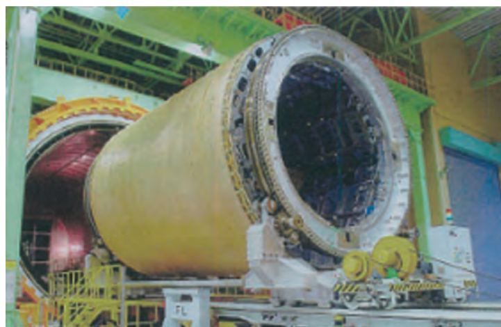
Fig. 3 Forward fuselage cured in an autoclave
