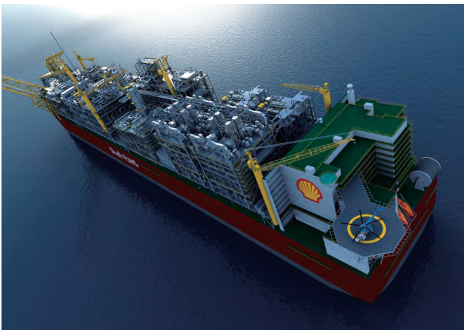
Fig. 3 Shell's Prelude FLNG fitted with seven 220 t/h boilers
