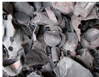
(b) Material recycled with magnetic separator
