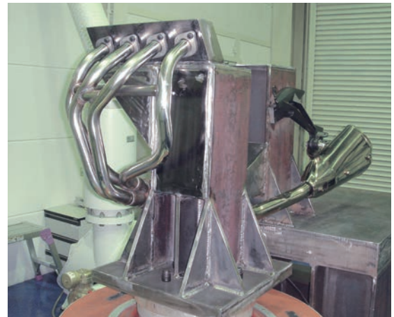
Fig. 7 Vibration test for exhaust system
