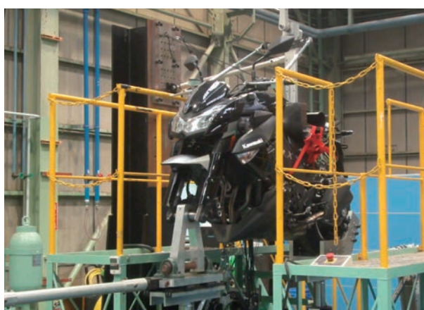
Fig. 12 Durability test using road simulator
