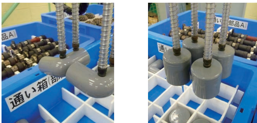
Fig. 10 Holding by suction
