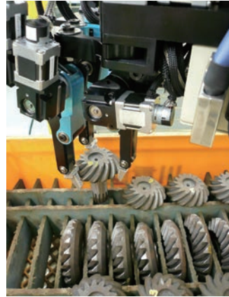
Fig. 2 Earlier version of the humanoid hand (2007)
