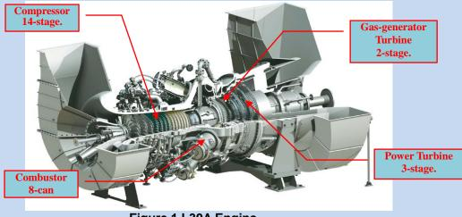
Figure.1 L30A Engine
