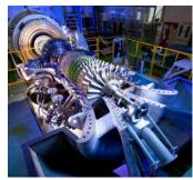
made-in-Japan, high-efficiency gas turbine "L30A"
