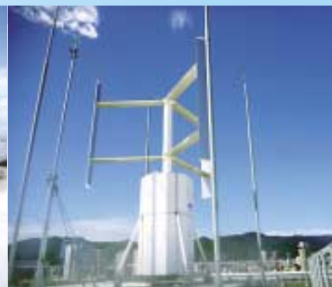
The vertical-axis wind power generation system is able to generate electric power efficiently using wind from any direction.
