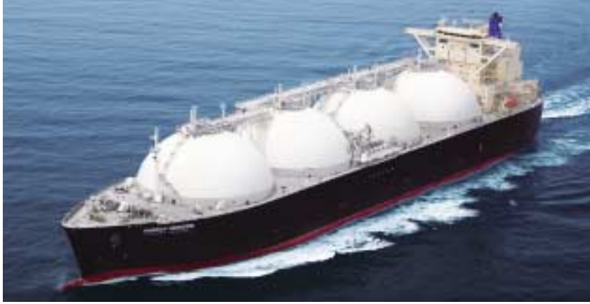
The versatile next-generation LNG carrier Energy Horizon (illustration) measures 300 m in length overall, 52.0 m in breadth and 11.5 m in draft (full draft: 11.9 m).
