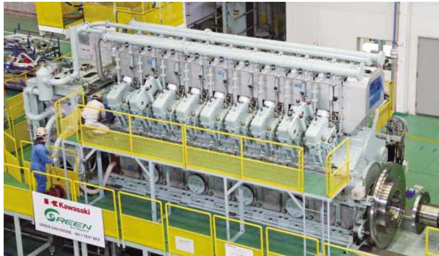
The Green Gas Engine. Having attained the world's highest generating efficiency of 49.0%, Kawasaki is continuing efforts to reach 50%.
