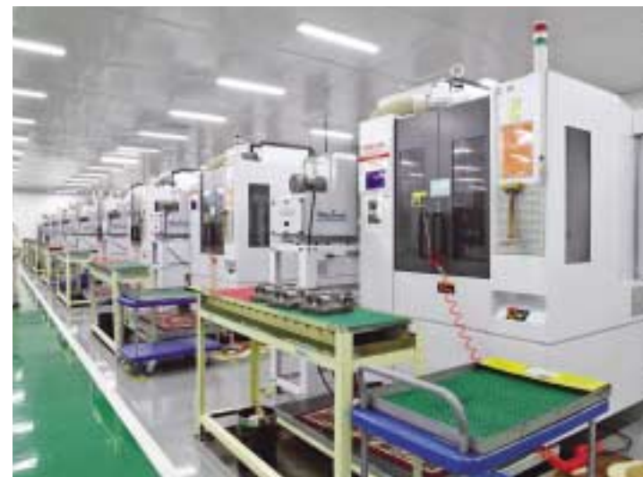
Machining centers (multifunctional numerically controlled machine tools) from Japan are used in the processing shop of the new plant.
