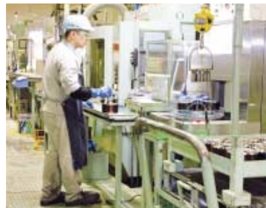
Cylinders for hydraulic equipment are inspected for the slightest imperfection.
