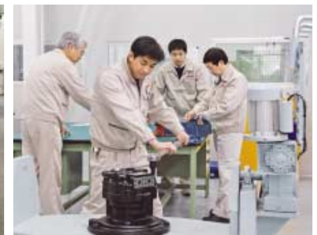
Overhauling hydraulic equipment at Kawasaki Precision Machinery Trading (Shanghai) Co., Ltd.'s Customer Service Center.
