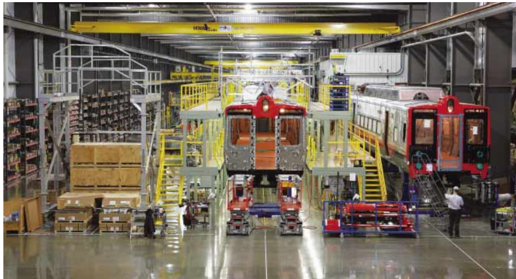
M-8 train cars at the end of the new rail car body production line, built to meet growing demand.
