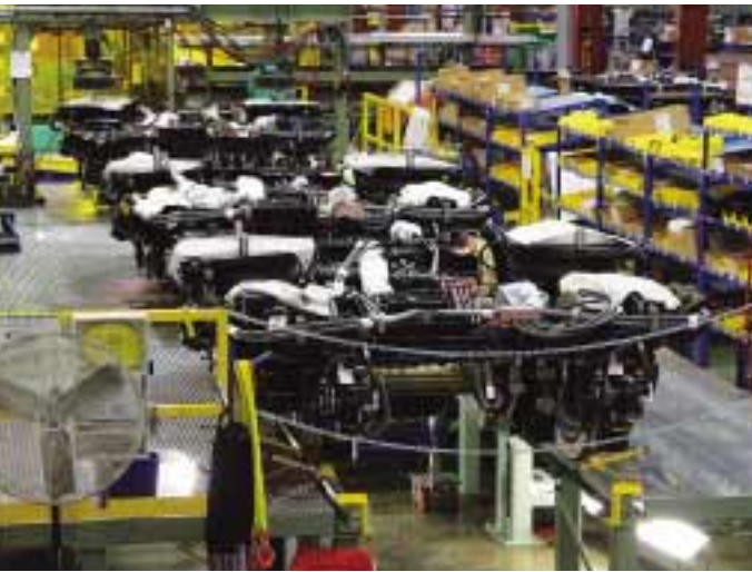
Assembling the very large bogies of the M-8, one of the largest commuter trains by width and length.
