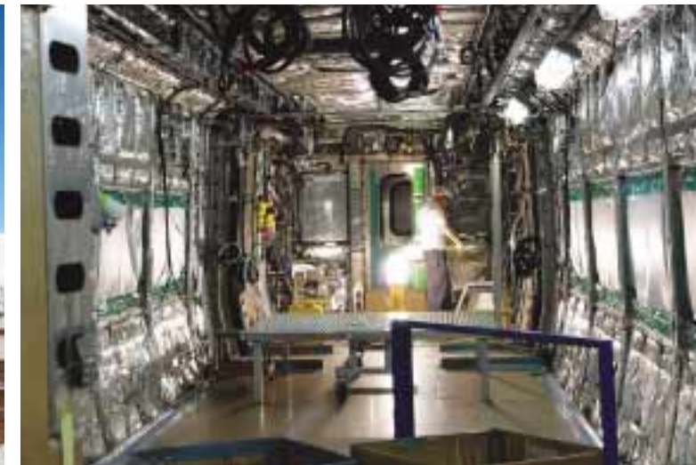
One by one, air ducts, door pockets, seats and various other components are installed inside the car. The rail car is put to the test at every step.
