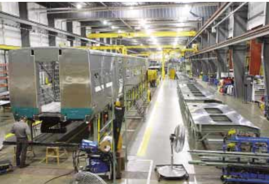
After adding two sides and the roof, it's beginning to look more like a train.
