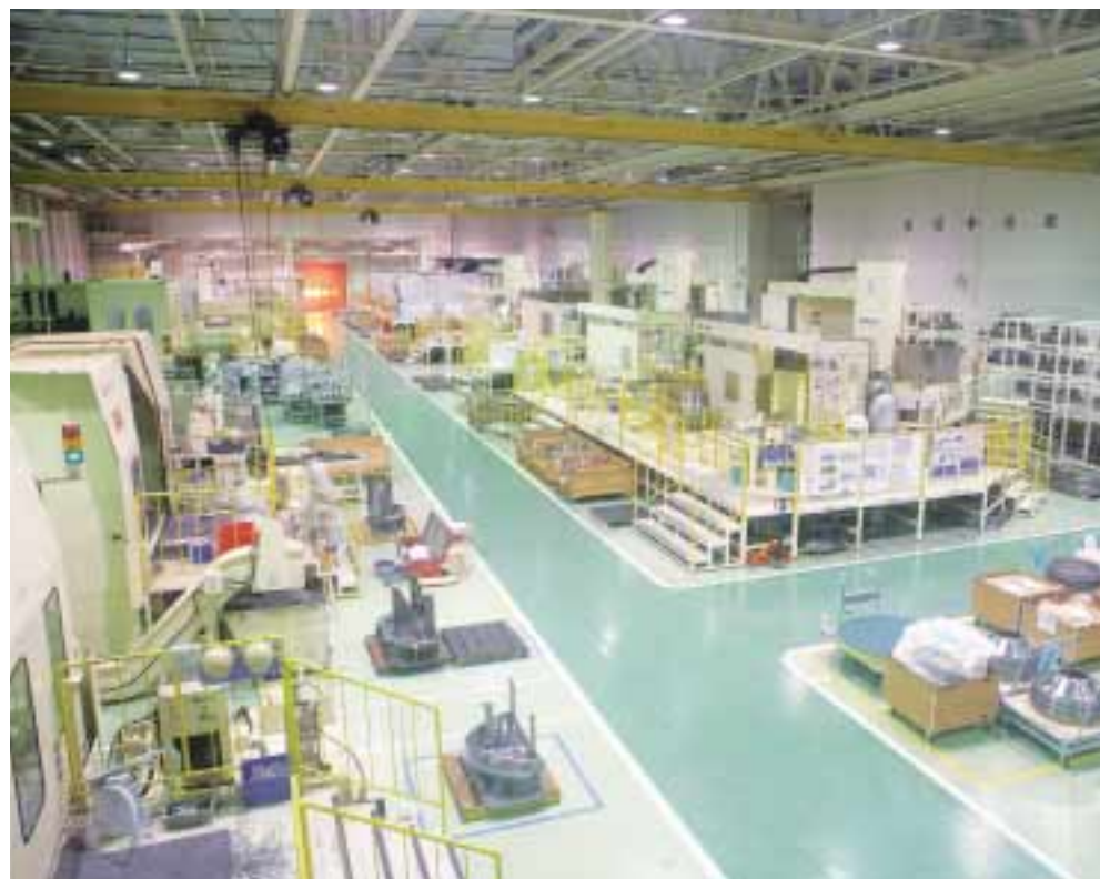
The Seishin Works machining shop, built exclusively for the Trent 1000. The facility is home to state-of-the-art machining tools, including the latest NC machining centers, as well as a number of one-of-a-kind or unique machines.
