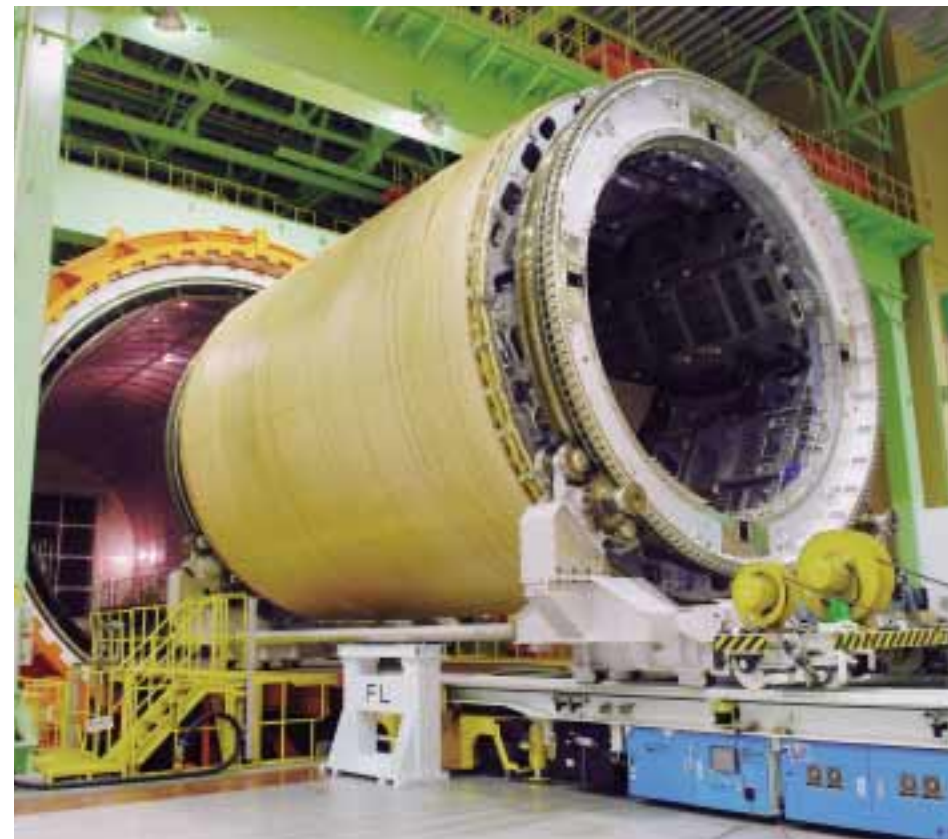
▶ A forward fuselage cured in one of the largest autoclaves in the world.
