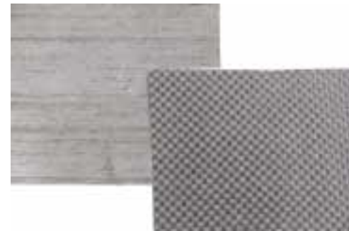
A sample of the carbon-fiber composite prepreg that, by weight, constitutes about 50% of the 787 airframe.
