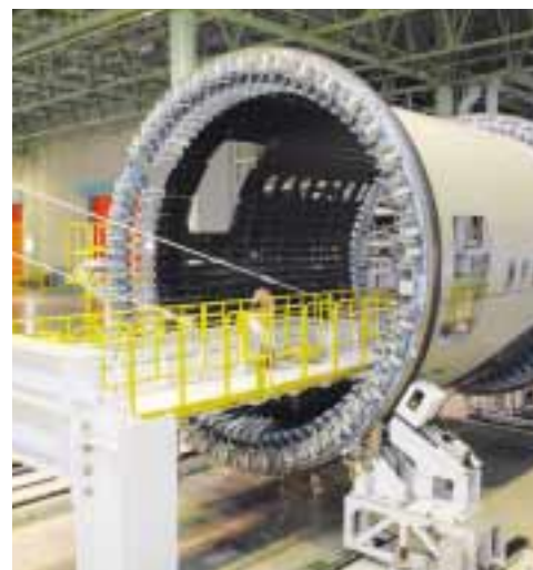
▶ A forward fuselage undergoes rigid inspection using ultrasonic non-destructive inspection equipment exclusively developed for the one-piece composite barrel.
