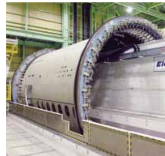
▶ A fastening machine automatically installs frames to a fuselage.
