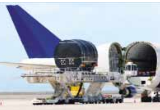
The forward fuselage produced by Kawasaki is transported to the U.S. by the Dreamlifter, Boeing's large cargo freighter.
