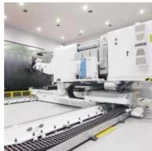
The state-of-the-art automatic fiber placement machine lays carbon-fiber composite material around a large cylindrical mold measuring 6 m in diameter.
