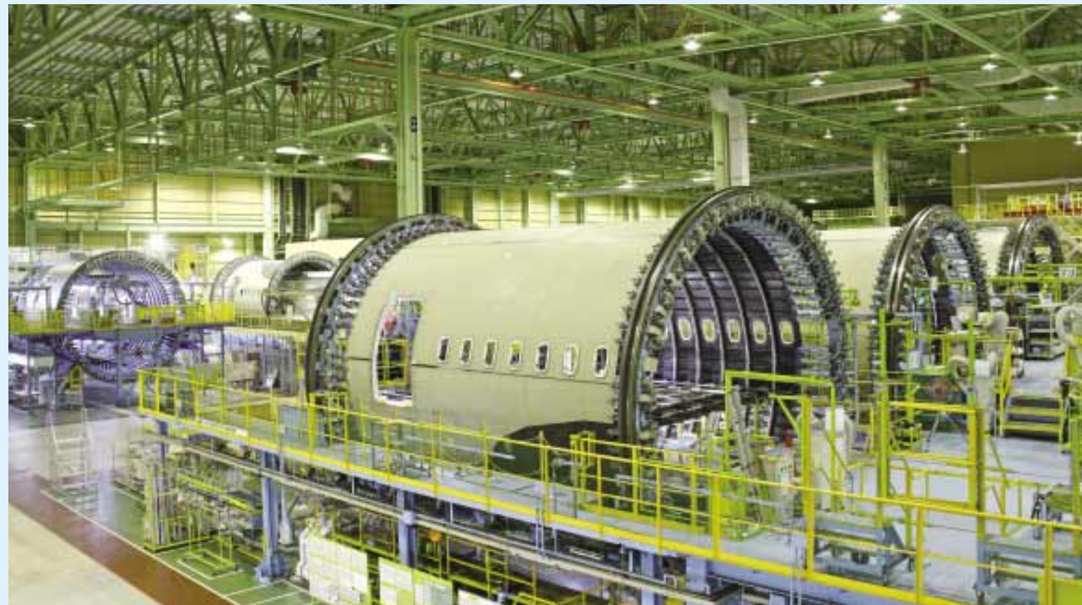
787 forward fuselages on the 787 North Plant's assembly stage (Nagoya Works 1).
