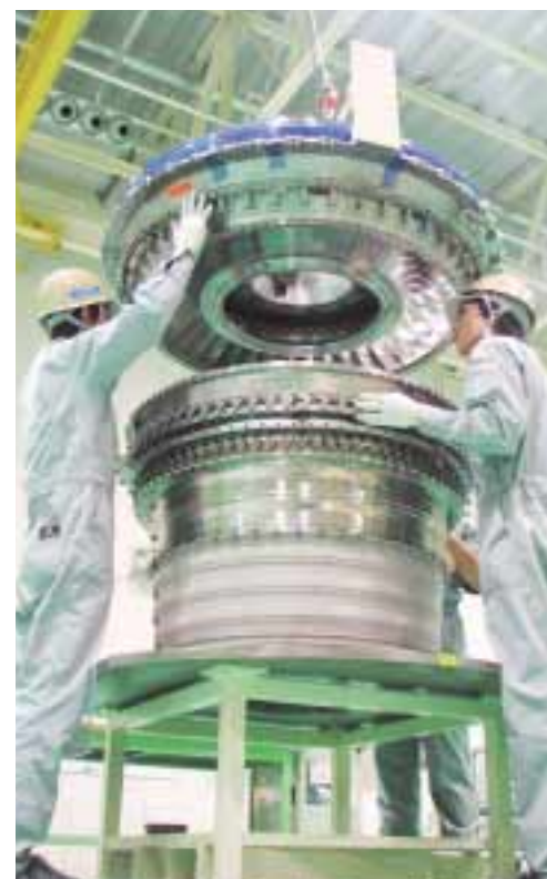
Assembly of the intermediate pressure compressor (IPC) module consists mostly of ultraprecision parts machined with micrometer accuracy.
