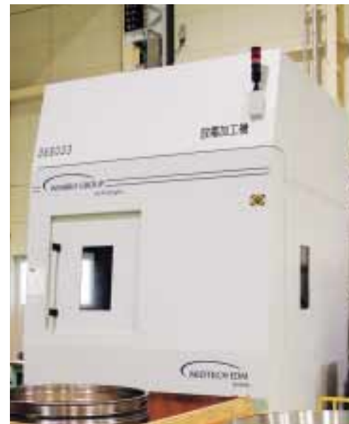
The world's only high-speed electrical discharge holing machine drills holes to exact specifications.
