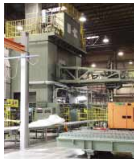
A huge SMC press machine, with a Jet Ski body moving on to the next process.
