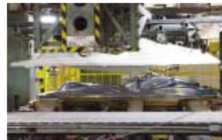
A Jet Ski body is formed via an SMC press.
