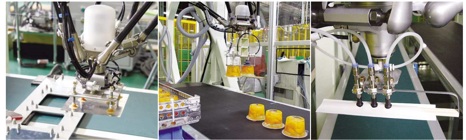
The robot can pick up objects of various sizes, either soft or hard, such as solar panels (left), food products like these containers of orange gelatin (center), and disposable chopsticks packaged in paper sleeves (right).
