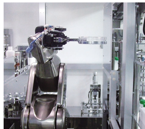
▶ All normal operations performed by the self-contained system's clean robot ensure a class 100 clean environment.
