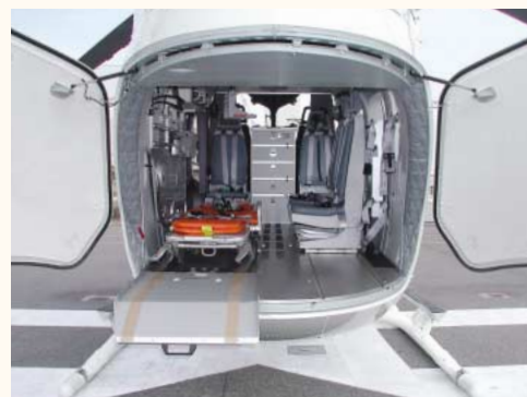
Large rear hatch with clamshell door.
