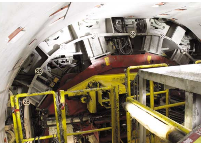
The shield machine excavates the tunnel face. The soil is hidden from view behind the machine.
