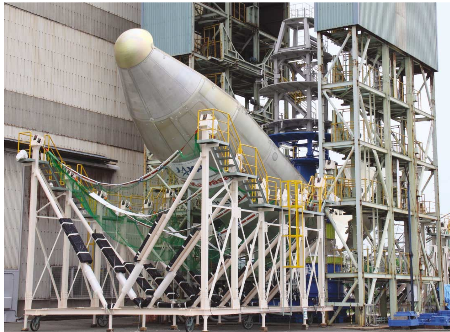
The 5S-H splits into halves upon detonation.
