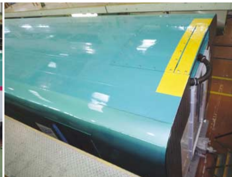
Rooftop components are completely encased.
