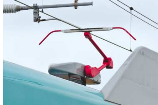
A low-noise pantograph fitted with an acoustic insulation panel minimizes environmental noise when operating at speeds up to 320 kph. (Photo courtesy of JR East.)
