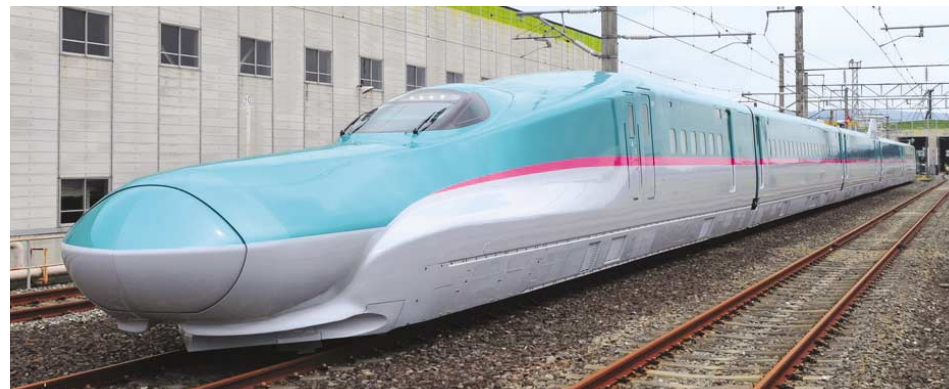
A sleek carbody featuring bogie shrouds installed on the lower section.
