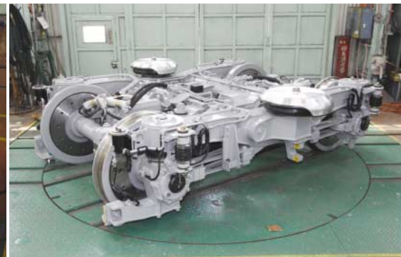
Bogie developed with a focus on safety, stability and minimal weight.
