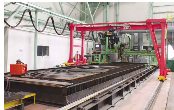
Steel plates are automatically cut to make tubes that house a screw propeller.
