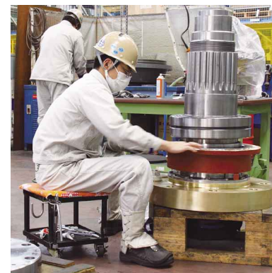
▶ The bevel gears are fine tuned so they mesh together perfectly.
