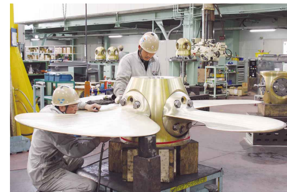
▶ The screw propeller (cast copper alloy) is assembled. Since it's a variable pitch propeller, the blades can be angled at different degrees.
