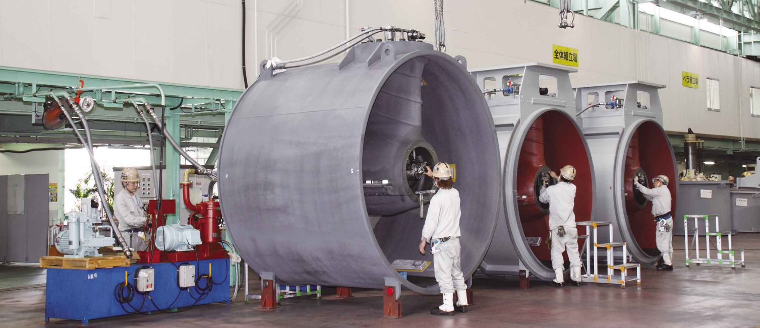
Side thrusters are put through a series of tough tests before they are ready for shipment.
