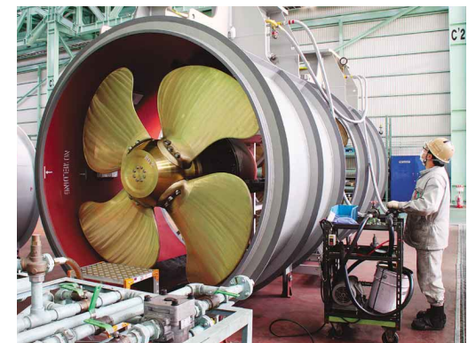
▶ The gear case is checked for oil leaks. The finished product is then put through rigorous tests before it's packaged and shipped.
