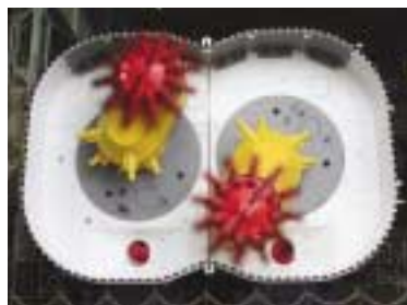
Cutter heads rotate as they turn on the revolving drum.
