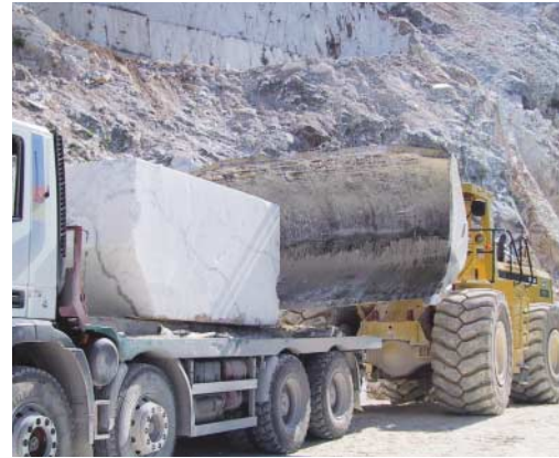
A wheel loader loads a marble block onto a dump truck, which will transport it to workshops in and around Carrara to be processed into high-grade interior building materials.
