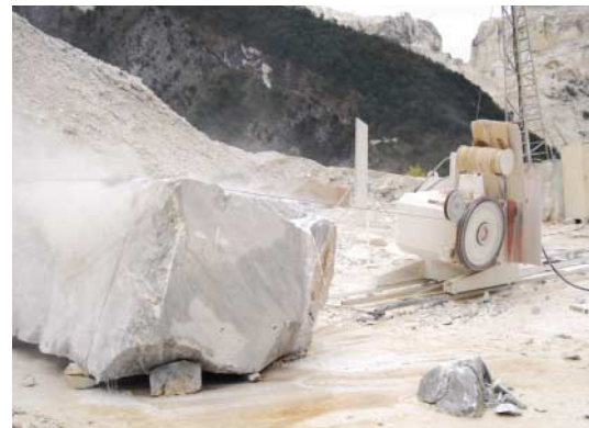
Excavated marble is cut into slabs with a wire saw.
