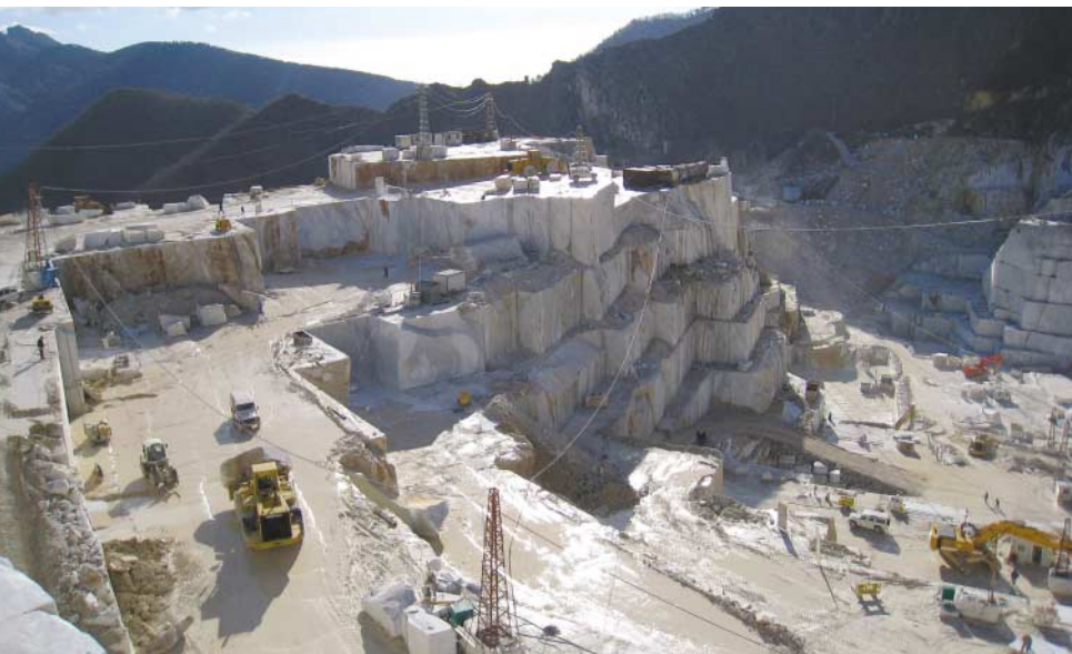
The quarry face is cut in steps (benches).
