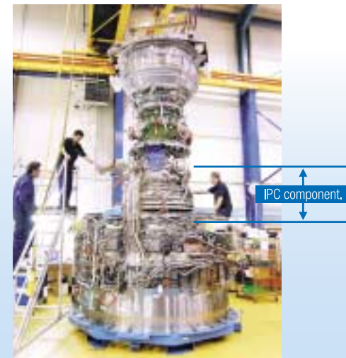
The IPC module is installed in this section of the Trent 1000. (Photo taken at the Rolls-Royce plant in Derby, U.K.)
