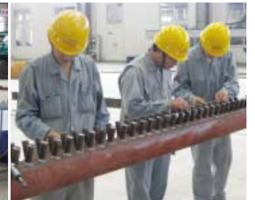
Welded boiler pipe joints are visually inspected.
