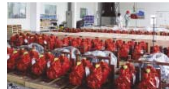
KPMC's core product, hydraulic pumps for 20 ton class excavators, ready to be shipped.
