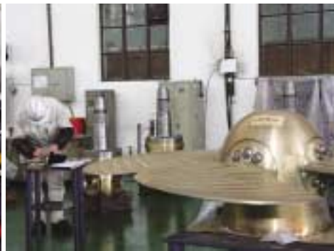
Getting ready to mount a propeller onto a side thruster.
