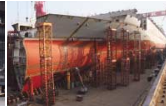
Block units are assembled into a ship on the dock.
