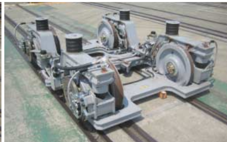
The middle bogie is axleless. The middle car's center aisle is positioned between the bogie wheels.
