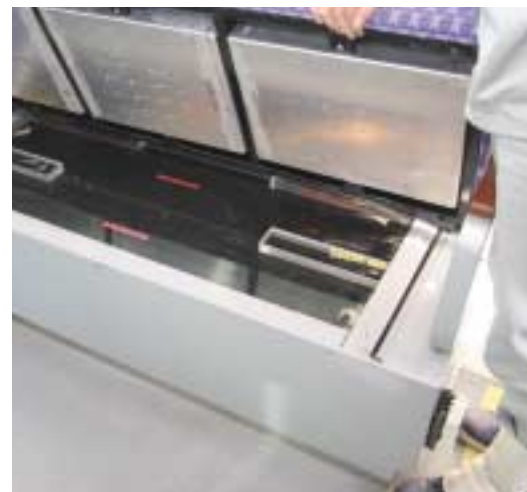
Kawasaki's proprietary Gigacell battery is installed under the seat.
