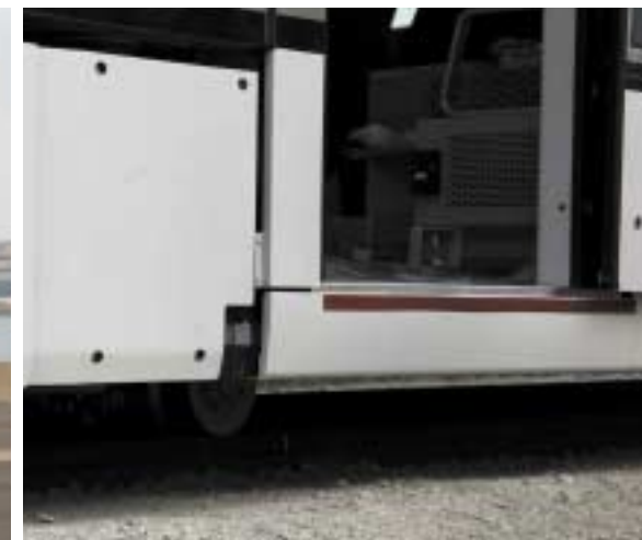
The door is only 330 mm off the ground, less than half of a conventional tram's height, making it universally accessible.
