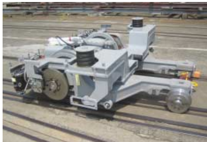
In the leading bogie, the driving wheels are on the left. The low-floor passenger cabin is installed above the smaller wheels on the right.
