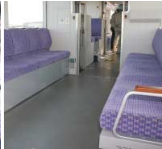
Employment of a compact bogie and mounting of electric devices on the roof allows SWIMO to have all-flat floors at both ends of the passenger cabins, and therefore, flexible seat arrangements.
