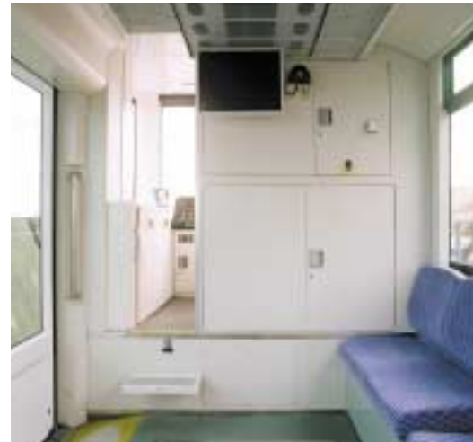
The low-floor design extends from the passenger cabins all the way to the operator's cab.
