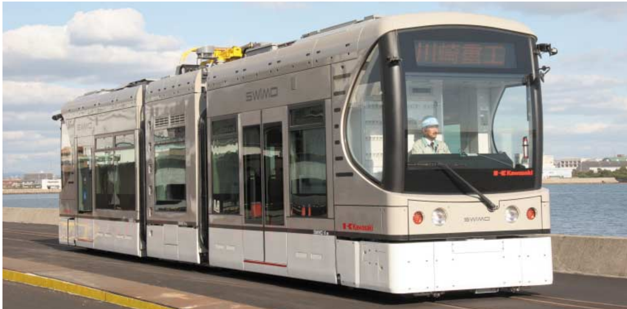
Testing of SWIMO's battery performance was conducted at a 1,600 m non-electrified test track at the Harima Works.
