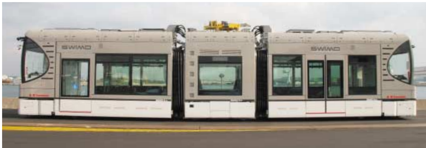
The SWIMO's profile. Its innovative 3-car, 3-bogie structure, with newly developed, compact bogies placed in the middle and at both ends, is a world's first.
