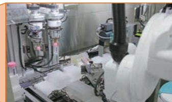
A robot performing opening and dispensing of specimens. Using robots for the process, which poses a high risk of infection, contributes greatly to reducing the burden on healthcare professionals.
