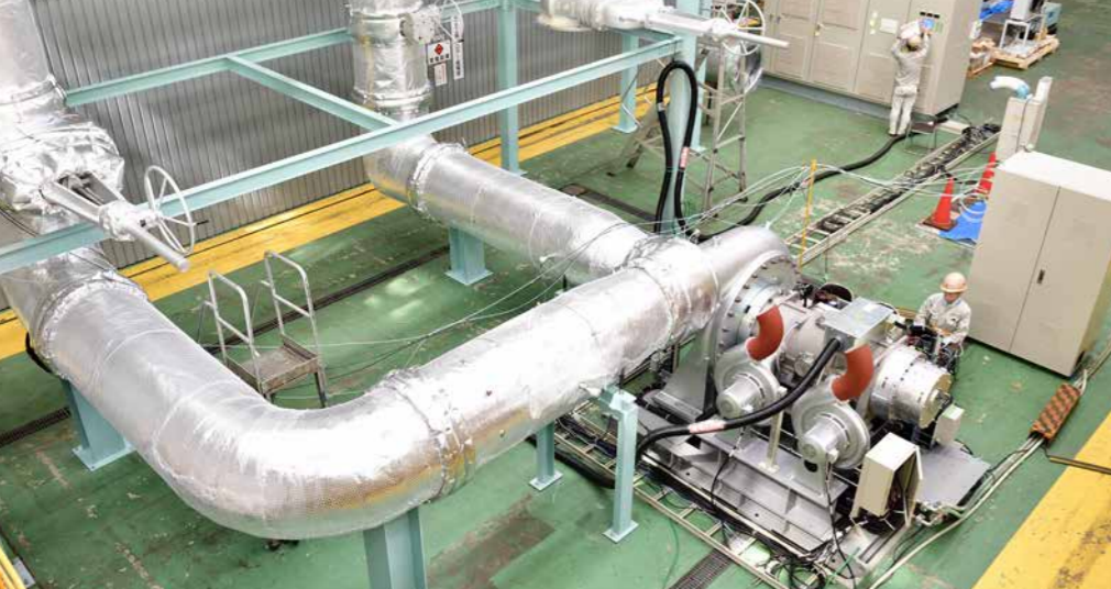
A Mega MAG Turbo M55 going through a final pre-shipping test at Kawasaki's Kobe Works. This unit is for a sewage treatment plant in Russia.
