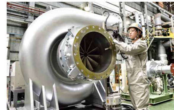
(Above) The M55 sits to the rear of the photo. The equipment in the foreground is the M25. In 2007, Kawasaki introduced the MAG Turbo, the components and parts of which are all Kawasaki-made. Since that model is considered the “second-generation” blower, the Mega MAG Turbo is technically the third generation. (Left) The Mega MAG Turbo being assembled. The fan-shaped objects inside the intake opening are inlet guide vanes.
